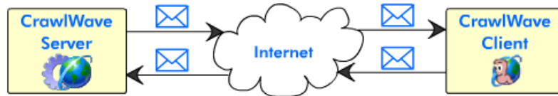
Fig. 2. XML messages between the client and the server of the CrawlWave
